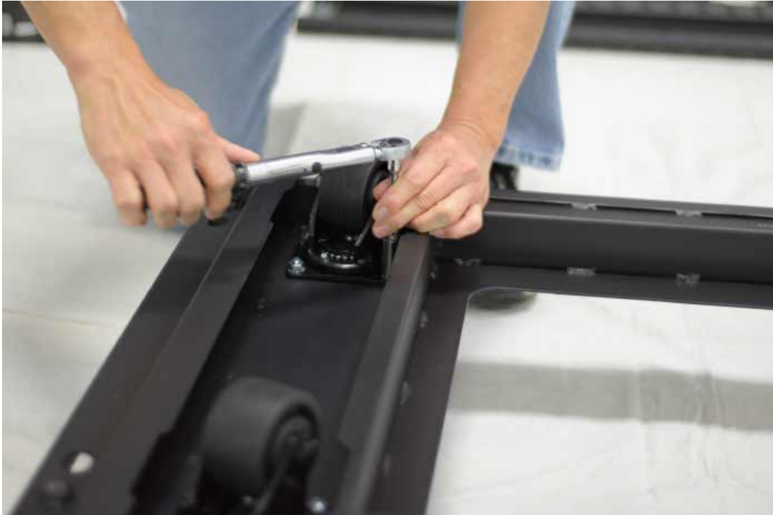
Torque Swivel Caster M8 Nuts
